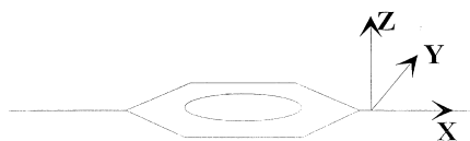
Figure 16 Diagram showing the three main axes of the chemical shift tensor for the unprotonated aromatic carbons on the phenyl ring in PET
